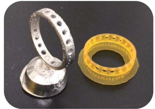
3D Printed Molding Examples Using UV-Curable 3D Resins
