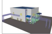
Conceptual drawing of the small-scale pilot plant for pharmaceutical intermediates in Fukuchiyama
